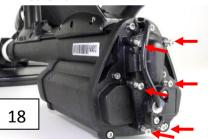
20. Connect Endcap and Battery Pack <u>then check and test the</u> F3 UXO Detector.
