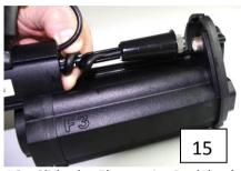
16. Slide the Electronics Pack back into place, replace two screws.
