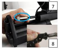
9. Remove the Coil Retainer.
